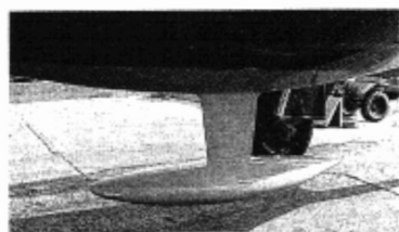
Bottom left: The Canard bulb fitted to Scoundrel in 1989. With this arrangement she won the British Open Championship in 1991 in convincing style.
